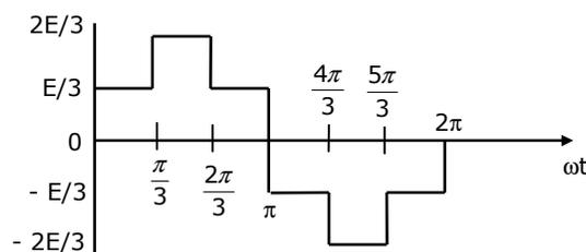
(P) single phase fully controlled ac-dc converter
