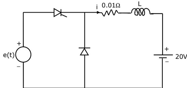
19. A line commutated a.c. to d.c. converter is shown in figure. It operates from a three-phase, 50 Hz, 580 V (line-to-line) supply. It supplies a load current,  $I_o$  of 3464 A. Assume  $I_o$  to be ripple free and neglect source impedance.
