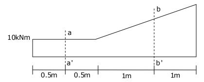
The shear force at sections aa' and bb' respectively are of the magnitude
