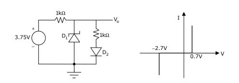
38. The transfer characteristics of the circuit drawn below is observed on an oscilloscope used in XY mode. The display on the oscilloscope is shown on the right hand side. V,- is connected to the X input with a setting of 0.5 V/div, and  $V_0$  is connected to the Y input with a setting of 2 V/div. The beam is positioned at the origin when V, is zero.
