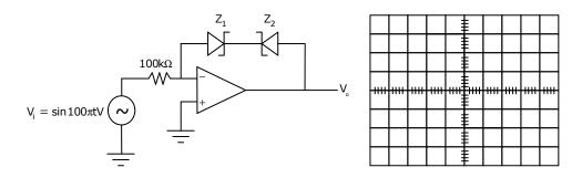
Assuming that the op-amp is ideal and the Zener diodes have forward biased voltage drop of 0.7 V, the values of reverse break-down voltages of Z1 and Z2 are, respectively,
