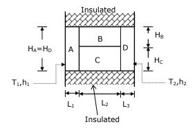
The dimensions are:  $H_A=H_D=3m$ ,  $H_B=H_C=1.5~m$ ,  $L_1=L_3=0.05m$ ,  $L_2=0.1~m$  The thermal conductivity of the materials are:  $K_A=K_D=50~W/m$ -K,  $K_B=10W/m$ -k,  $K_C=1~W/m$ -k.
