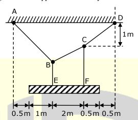
Determine the tension force in segment AB at this cable (correct to 1 decimal place). Assume the cable ABCD, BE and CF are weightless
