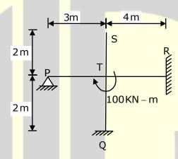
Find the magnitude of the B.M. at Q (in kN-m) due to given loading?
