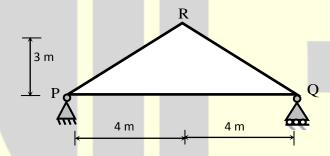
The magnitude of vertical displacement of joint R (in mm) is \_\_\_\_\_\_.
