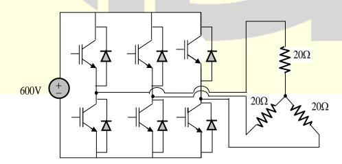
For a star connected resistive load of 20  $\Omega\,$  per phase, the load power for  $120^o$  device conduction, in kW is
