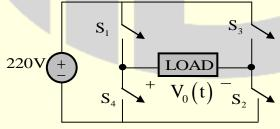
The RMS value of the fundamental component of  $V_o(t)$  in volts is \_\_\_\_\_\_
