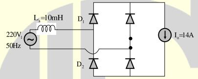
The load draws a constant current  $I_o = 14A$ . The conduction angle of the diode  $D_1$  in degrees is
