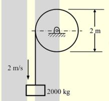
The mass moment of inertia of the drum is 150 kg-m<sup>2</sup>. On applying the brake, the mass is brought to rest in a distance of 0.5 m. The energy absorbed by the brake (in kJ) is
