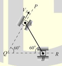
The sliders can slide along *QP* and *QR*. If the velocity *VA* of the slider at *A* is 2 m/s, the velocity of the midpoint of the rod at this instant is \_\_\_\_\_ m/s.
