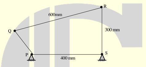
For the mechanism to be crank-rocker mechanism, the length of the link PQ can be
