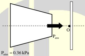
The inlet and outlet area of the nozzle are 0.1 m<sup>2</sup> and 0.02 m<sup>2</sup>, respectively. Take air density as constant and equal to 1.2 kg/m<sup>3</sup>. If the inlet gauge pressure of air is 0.36 kPa, the gauge pressure at point O on the plate is \_\_\_\_\_kPa (round off to two decimal places).
