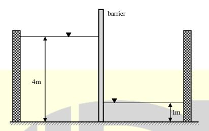
Taking the density of water as  $1000 \text{ kg/m}^3$ , and the acceleration due to gravity as  $10 \text{ m/s}^2$ , the maximum absolute bending moment developed in the cantilever is \_\_\_\_\_kN-m (round off to the nearest integer).
