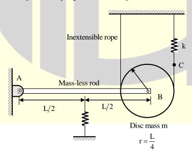
There is no slip between the rope and the pulley. The system is in static equilibrium in the configuration shown in the figure and the rope is always taut.
