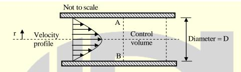
The rate of kinetic energy (in J/s) at the control surface A-B, as shown in the figure, is proportional to  $D^n$ . The value of n is \_\_\_\_\_\_\_.
