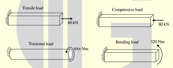
Which specimens(s) will fail due to the applied load as per maximum shear stress theory?
