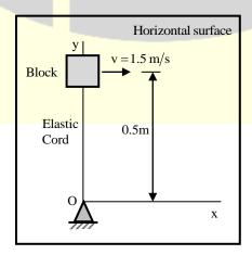
The cord hinged at O is initially unstretched and always remains elastic. The block is given a velocity v of 1.5 m/s perpendicular to the cord. The magnitude of velocity in m/s of the block at the instant the cord is stretched by 0.4 m is
