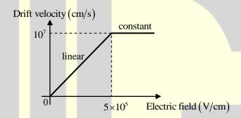
The semiconductor has a uniform electron concentration of  $n = 1 \times 10^{16} \text{ cm}^{-3}$  and electronic charge  $q = 1.6 \times 10^{-19} \text{ C}$ . If a bias of 5V is applied across a 1  $\mu m$  region of this semiconductor, the resulting current density in this region, in  $kA/cm^2$ , is
