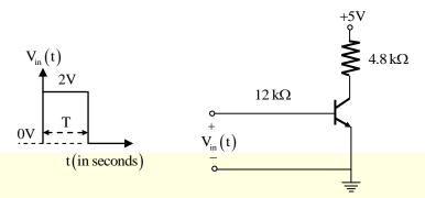
For the input  $V_{in}(t)$  as shown in the figure, the transistor switches between the cut-off and saturation regions of operation, when T is large. Assume collector-to-emitter voltage saturation  $V_{CE(sat)} = 0.2V$  and base-to-emitter voltage  $V_{BE} = 0.7V$ . The minimum value of the common-base current gain ( $\alpha$ ) of the transistor for the switching should be \_\_\_\_\_.
