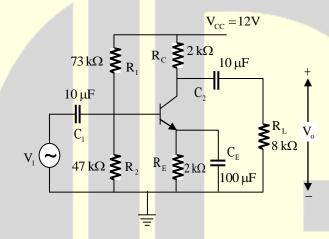
Given that  $V_T = 25 \text{mV}$ ,  $V_{BE} = 0.7 \text{V}$ , and the BJT output resistance  $r_0$  is practically infinite. Under these conditions, the midband voltage gain magnitude  $A_V = \left| V_o / V_i \right| V / V$ , is \_\_\_\_\_\_.
