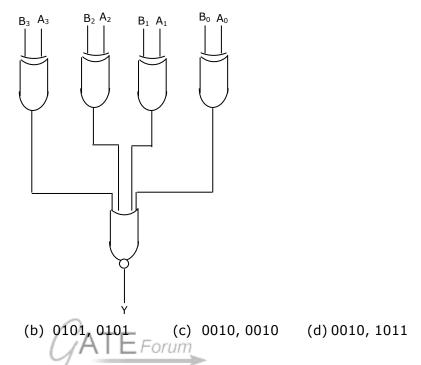
68. The digital circuit shown in figure generates a modified clock pulse at the output. Choose the correct output waveform form the options given below.
