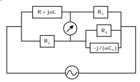
(A)  $R = R_2 R_3 / R_4$ ,  $L = C_4 R_2 R_3$
