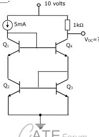
1.21. In figure, both transistors are identical and have a high value of beta. Take the dc base-emitter voltage drop as 0.7 volt and KT/q = 25 mV. The small signal low frequency voltage gain  $(V_o/V_i)$  is equal to \_\_\_\_\_
