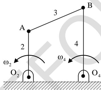
The magnitude of the angular speed of the output link 4 is  $\omega_4$  at the instant when link 2 makes an angle of  $90^\circ$  with  $O_2O_4$  as shown. The ratio  $\frac{\omega_4}{\omega_2}$  is \_\_\_\_\_ (round off to two decimal places).
