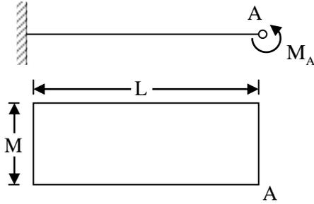
$$EI = 200 \text{ N-m}^2, \quad L = 1.0 \text{ mts}, \quad M_A = 1.0 \text{ N-mts}$$
