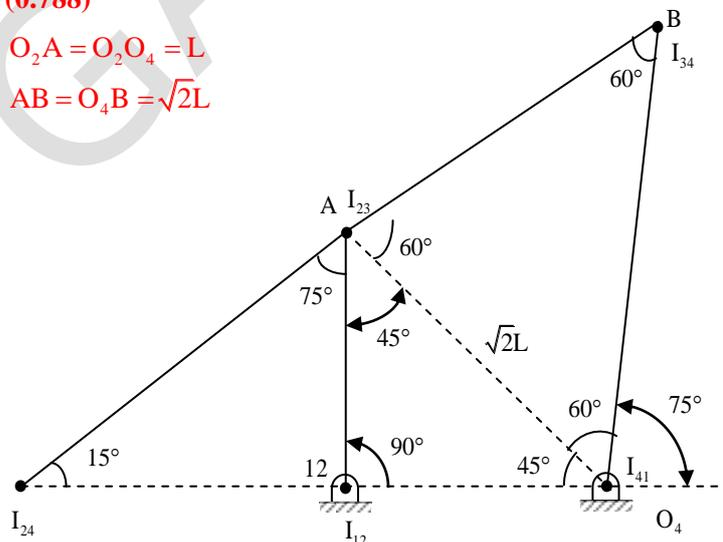
$$I_{24} I_{12} \omega_2 = I_{24} I_{41} \omega_4$$
