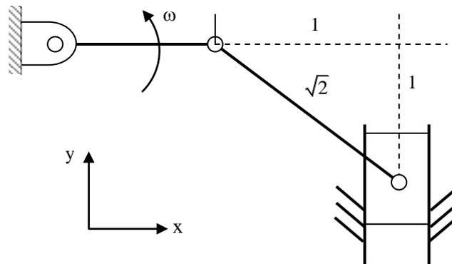
Using exact analysis. The acceleration of the slider in the  $y$ -direction, at the instant shown, where the crank is parallel to  $x$ -axis, is given by
