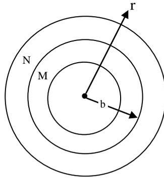
At the radial location  $r=b$ , there will be a contact pressure and element at interface of cylinder M and N the radial displacement will be same
