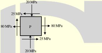
By how much angle  $(\theta)$  in degrees the stress element should be rotated in order to get the planes of maximum shear stress?
