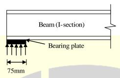
As per IS: 800-2007, the web bearing strength (in kN, round off to 2 decimal places) of the beam is \_\_\_\_\_.
