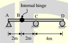
The relative positions of the two loads are not fixed. The maximum shear force (in kN, round off to the nearest integer) caused at the internal hinge B due to the two loads is \_\_\_\_\_.
