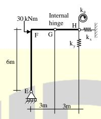
For the externally applied moment of 30 kNm at node F, the rotation (in degrees, round off to 3 decimals) observed in the rotational spring at node H is \_\_\_\_\_.
