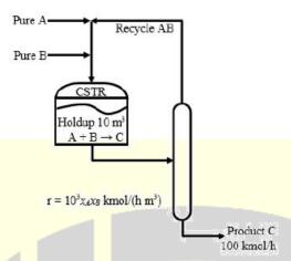
Other relevant information are provided in the figure. The mole fraction of B  $(x_B)$  in the reactor that minimizes the recycle rate is (rounded off to two decimal places).
