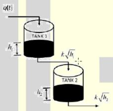
At steady state operation, the water inlet flow rate is  $q_{ss} = 16 \text{cm}^3 / \text{s}$ . The transfer function relating the deviation variables  $\tilde{h}_2$  (cm) to flow rate  $\tilde{q}$  (cm<sup>3</sup>/s) is
