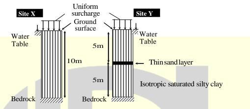
The silty clay layers at X and Y are identical. The thin sand layer at Y is continuous and free-draining with a very large discharge capacity. If primary consolidation at X is estimated to complete in 36 months, what would be the corresponding time for completion of primary consolidation at Y?
