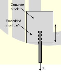
Let  $\sigma_b$  and  $\sigma_{st}$ , be the bond strength (between the bar and concrete) and the tensile strength of the bar, respectively. If the block is held in position and it is assumed that the material of the block does not fail, which of the following options represents the maximum value of P?
